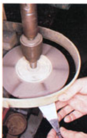
Even though I hold the tool under the rotating disc, I can see how the bevel is being sharpened from above. A strong light source from my vantage point helps me see the tool.
