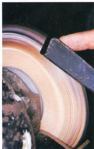
For the inside of the V, I use a special polishing wheel that matches the inside profile.
