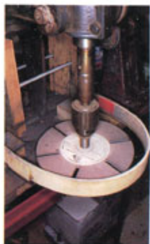
A horizontal grinding disc has slots that radiate out from the center. When I grind a tool, I hold it under the disc, which is held in a drill press.
