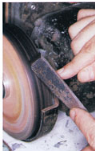
I use the same procedure of moving one side across the wheel at a time—the U shape last—on a polishing wheel.
