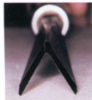
For the V tool to cut properly, it should have a U shape where the sides come together.
